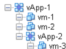
Figure 5 Example nested container structure
